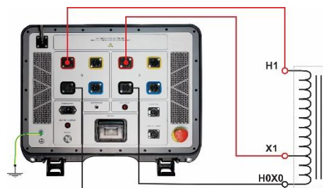
Connecting TWR-B to a single-phase autotransformer
