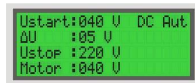
Figure 1. Setting up MTV test
