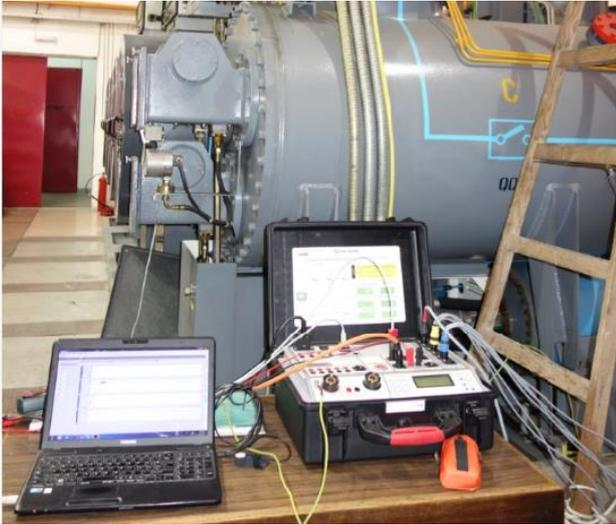
Figure 1. Circuit Breaker Analyzer CAT65
