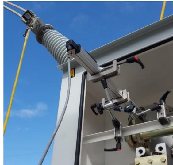
Figure 2. Linear transducer mounting example
