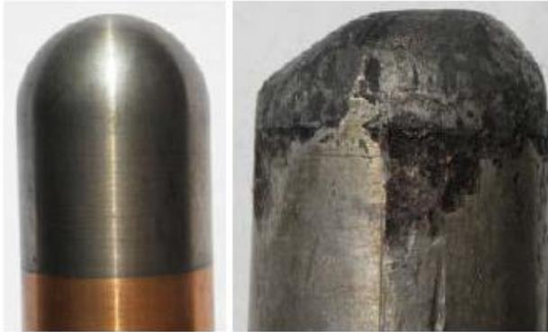
Figure 3. Arcing contacts: new (left) and worn (right)
