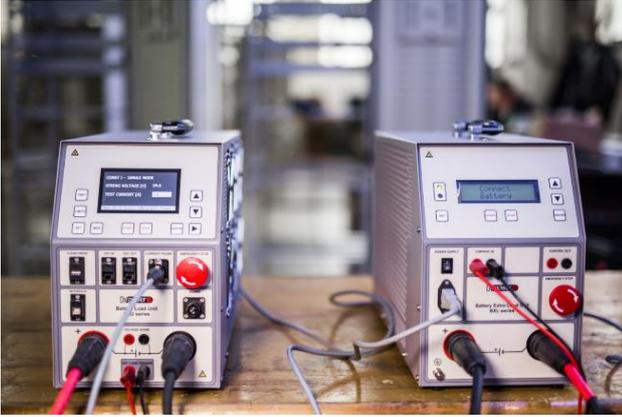
Using our BLU Series of instruments, the capacity test can be completed in a short time.
